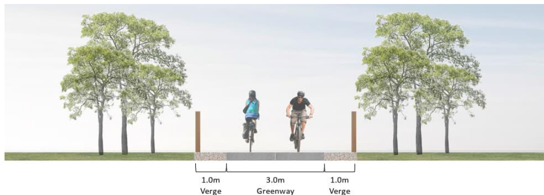
Figure 1-1 - Typical Cross Section of 3.00m Wide Greenway
